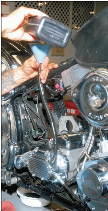
With the transmission buttoned up, it's time to add oil. Don't skimp on gear lube—use only the best.
