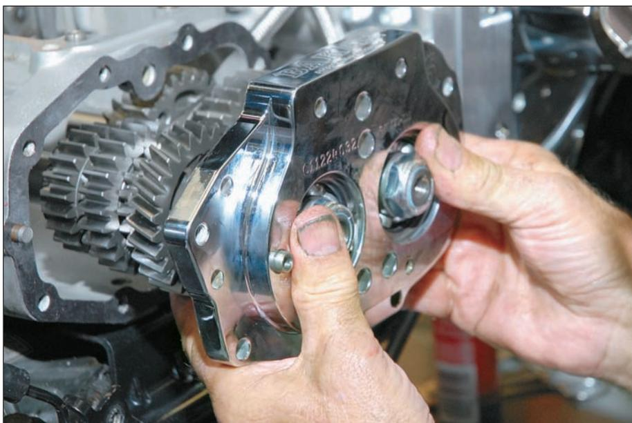
After the stock transmission is removed from the case, slip the Baker unit right back in. Don't forget the new cover gasket.
