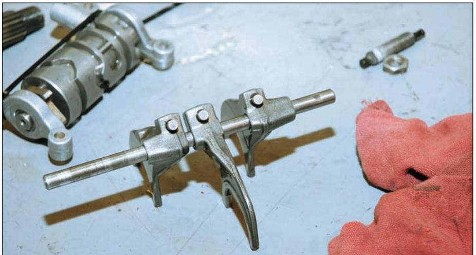
Posie trial-fits the Baker shift forks to the shaft before installing them. The Baker shift drum is seen at left.
