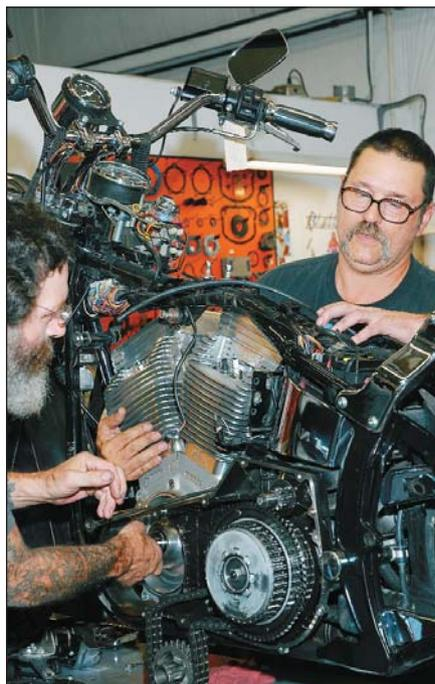
**Aligning the crankshaft with the primary assembly sometimes can be tricky. An assistant here is worth all the beer he wants to consume later. Emphasis on later.**
