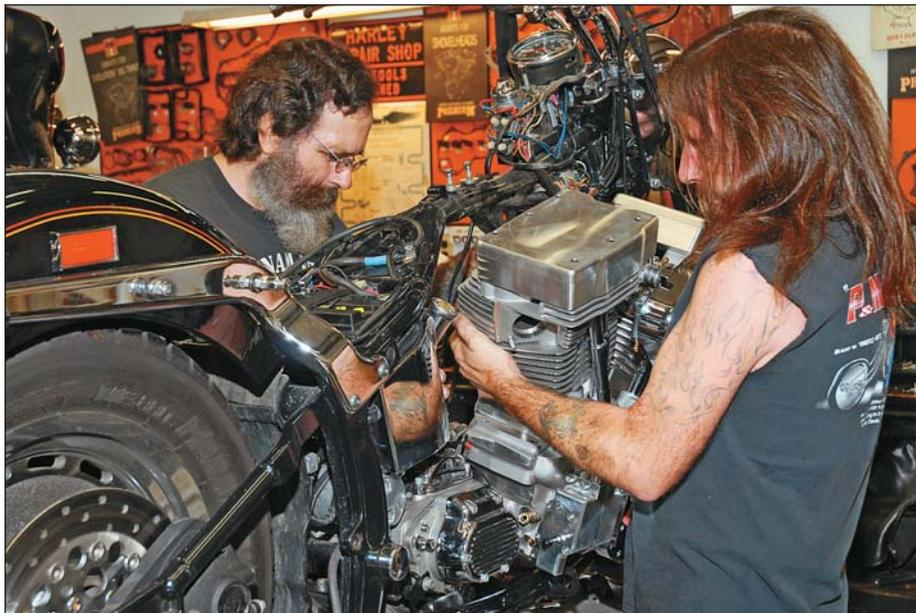
**Guiding the Delkron 120 into the frame takes patience, and sometimes a bit of grinding for clearance. Some frames have a tighter fit than others.**
