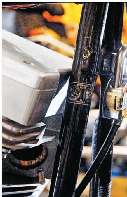
The front downtube clearance is tight on Softails with the Delkron 120. On rubber-mount frames for FLs and Dynas, the gap is much wider, so the engine can rock on its mounts.
