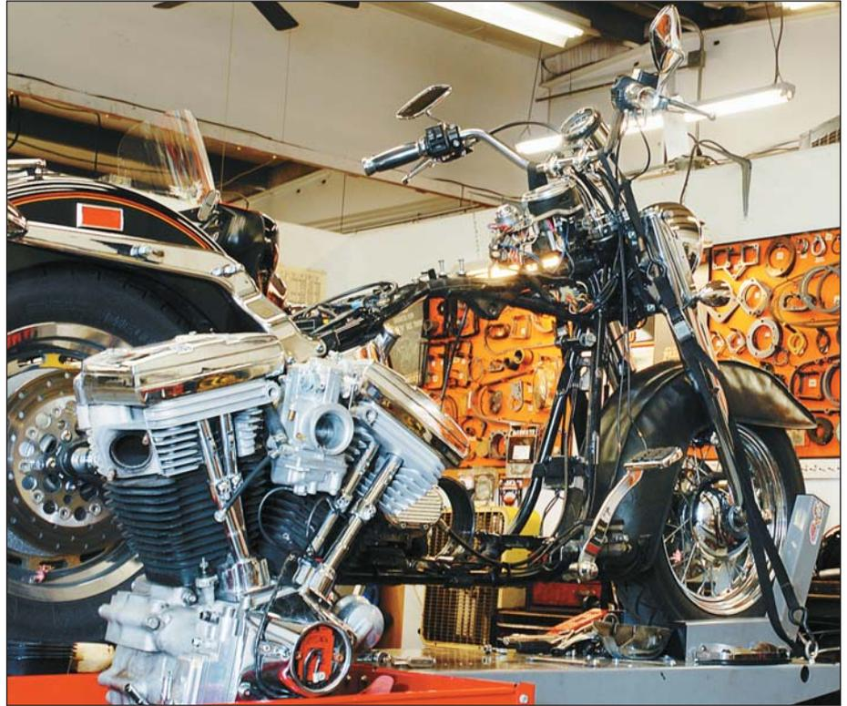
With the old heart (okay, engine) removed, the patient remains stable. Tying the bike down on a raised, level working surface makes the job easier.
