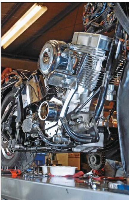
The Delkron engine is in the frame, but not yet bolted. This is the last chance to make sure everything fits right. Examine every angle before tightening nuts and bolts.
