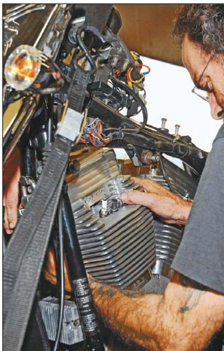
**Make sure all of the bike's electrical wires are out of the way when you install the Delkron 120. Pinching a wire now can mean hours of troubleshooting later.**
