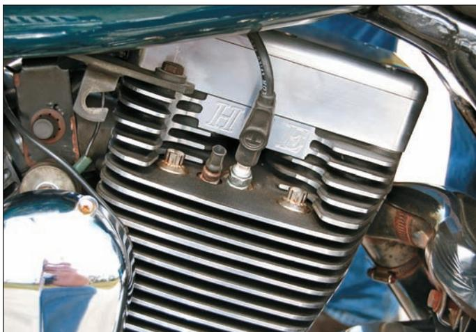
Dolecki, one of the crew from HSE, Inc. South. The ol' bag had a lot of get up and go, though, for an 18-year-old bike. That's because recently it had a heart transplant, in this case replacing its aging 80-cubic-inch, 45-horsepower, single-cam Evo (remember them?) for a new HSE 120. That's 120 as in 120 cubic inches, and that big mill served up a nice dose of roll-on power, too.
