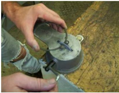
It is very important that the ring ends are square when installed into the cylinder bore. Ring end gaps that are not square will lead to incorrect ring end gaps that can lead to undesirable engine operation / function as well as irreparable engine damage.
