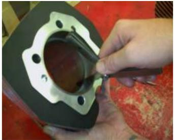
**<u>DO NOT</u>** round to the next lowest number ... example: .0165" to .016". It is better to be slightly larger with your ring end gap than smaller. Insufficient clearance on the compression rings can lead to "Ring Abutment" at operating temperature while under compression causing irreparable engine damage.
