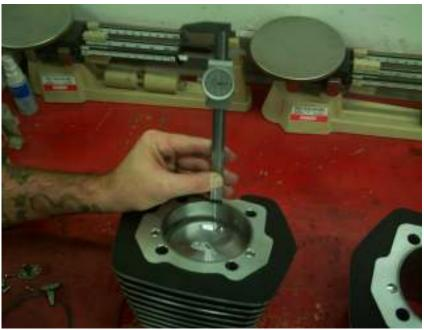
Correct top compression ring and secondary compression ring end gap is equal to .004" per inch of cylinder bore ... example: 4.125" x .004" = .0165" of ring end gap. Rounding this number to the next highest number is permissible ... example: .0165" rounds to .017"
